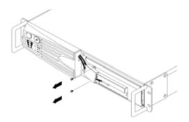
Remove the two retaining screws of the cable protection cover then remove the cover.
